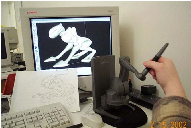
Student Tom Purcell using the FreeForm system with the PHANTOM Desktop haptic device to model “FrogDog”.
